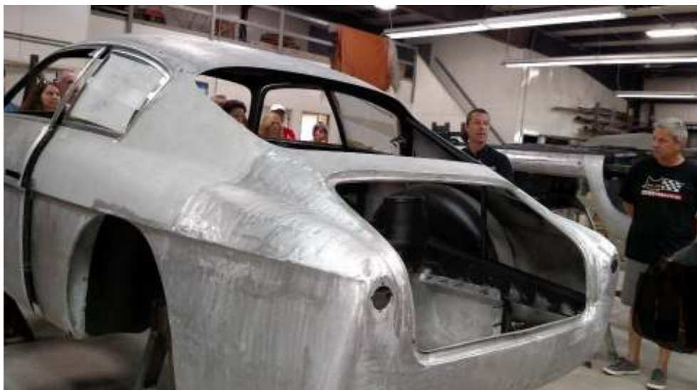
Dustiin Wetmore, center, discusses the body work being done on a Ferrari Zagato. Learn more about MPI at http://www.mpi-ferrari.com/index.html
